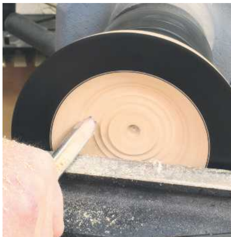
▲ Pic.11 Once the cut is started, work from the edge of the bowl to the centre. Take it down in stages, leaving some timber in the middle, which will be removed as you work down
